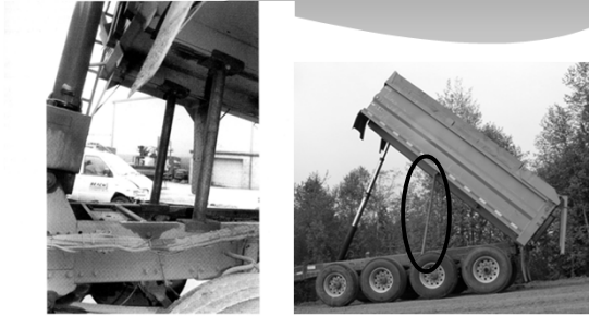
Figure 5.14 Prop (scotch) under raised body of tipper lorry. (Courtesy T E Beach Ltd) Ridley & Pearce, 2006
